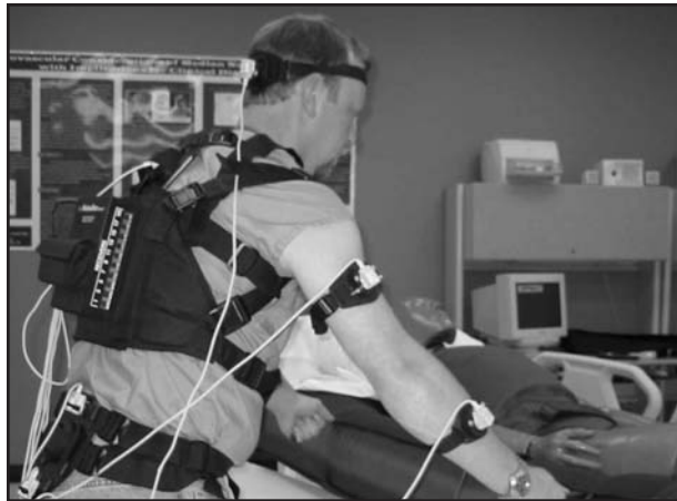
Figure 2. The study participant is performing a bed to stretcher lateral transfer task. Throughout execution of this task, postural demands were acquired through real-time measures of human motion using HumanTRAC (Gross, 1997).
